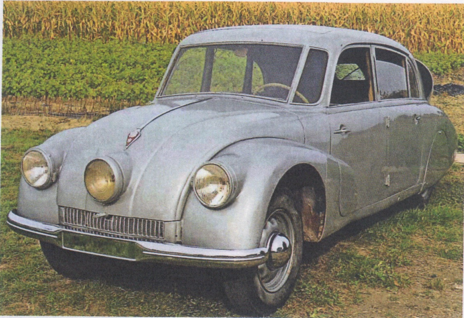
4a Tatra T87 has an air-cooled V8 mounted at the rear
