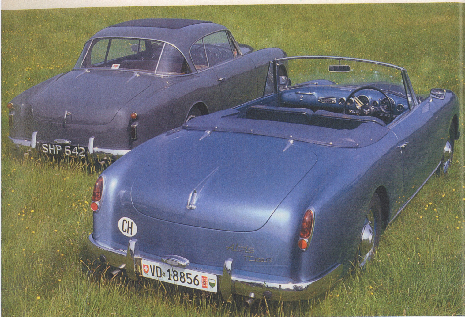
Above: differing tails on two TC108Gs; note Rolls lamps and handle strake on cabrio. Left: TC21 cabrio dash is as TA21 coupé's. Right: 'Panoramic', with new-for-1959 bonnet scoop
